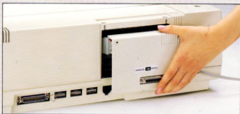
Back of printer showing parallel and serial interfaces
